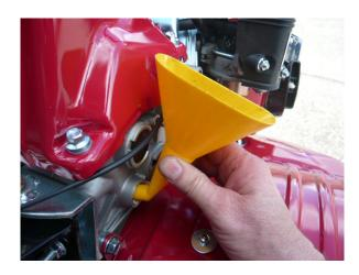
16. Fill the engine with oil up to the top of the threads in the filler hole using a small funnel. Use 10–40 sae
