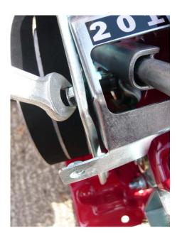
9. Install handlebars to top mounting plate section using 4 the bolts you removed in step 2 and tighten carefully.(do not over tighten into aluminium casting)
