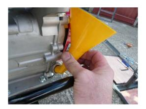
17. Fill the Air filter with oil up to the mark shown on clear cover. Use 10-40 sae
