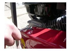
4. Remove 2 x bolts from gear selector bracket
