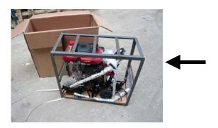
2. Undo and remove the 4 Handle bar securing bolts from top of mounting section and put to one side.
