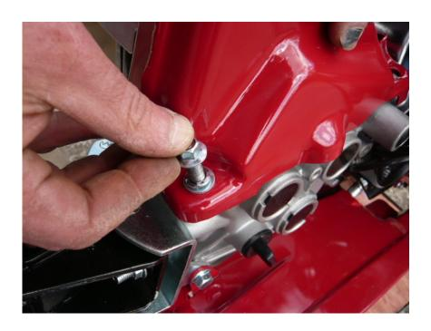
10.Install the L/Hand & R/Hand tine guards to the engine deck using lock nuts & bolts supplied in brown box. Step 1, 3 on each side.
