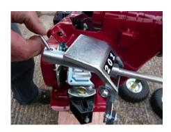
6. Locate gear selector stick onto male shaft and insert cotter pin through both using long nose pliers from the top of the machine.
