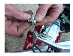
5. Remove Cotter Pin & split pin from connecting gear lever end
