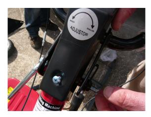
15.Fill gearbox with engine oil using a small funnel up to the threads in the filler hole. Use 10-40 sae
