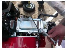
3. Remove tie wrap and bolts from drive belt cover and remove carefully.
