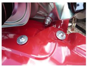
11.Install the tine guard support bracket to the underside of the guards using the 4 nuts, bots & washers supplied.
