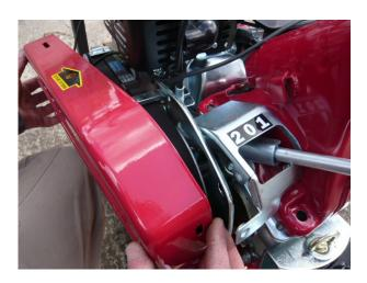
13. Attach handle bars to stem using the quick release handle
